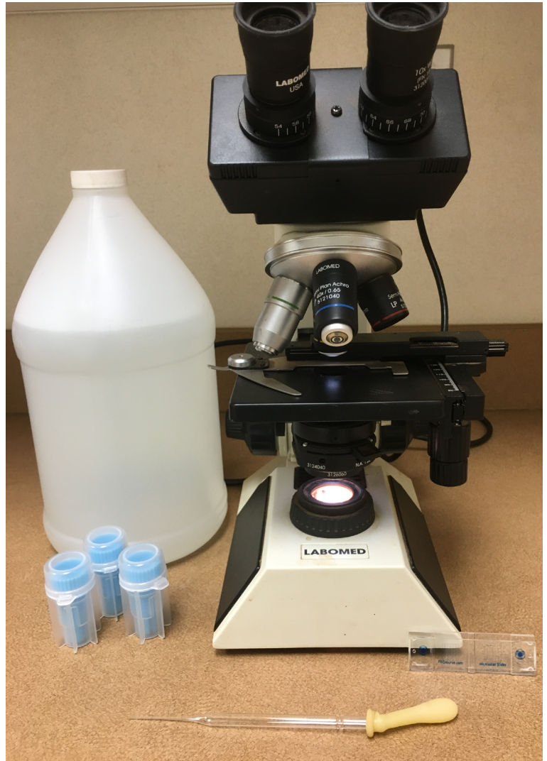
Figure 1. The basic supplies needed to perform a fecal egg count include a microscope capable of magnifying to 100X, a Mc-Master slide, a flotation solution that allows eggs to float to the top for ease of counting, pipette or eye droppers, fecal ova float containers or beakers (with mL lines for measuring), and a small scale capable of measuring in grams.
